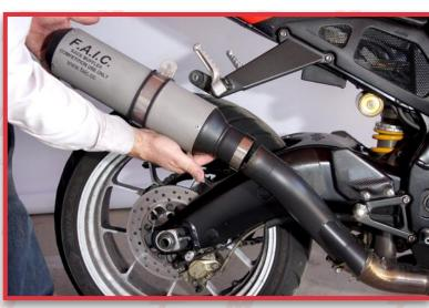
Step 6 (a): Install The Muffler Hanger (Direct Mounting To Stock Bracket)
