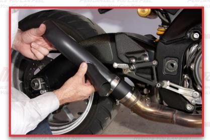
5. Tighten the Band Clamp securely to the Mid-Pipe.
